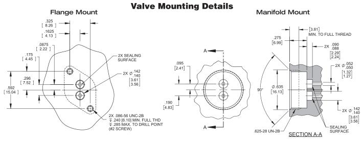
Reference Drawing Number LSIX1001540A for Mounting Details. Reference Drawing Number LSIX1001530A for Mounting Details. Unless otherwise specified, dimensions are in inches [mm]. Drawings are not to scale.
