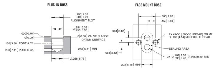
Boss geometries and dimensions shown above are for reference only. All dimensions are in inches [mm]. Reference Drawing Number LCFX0300250B for complete Plug-In Boss specifications and Drawing Number LFIX1002050A for complete Face Mount Boss specifications.
