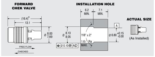
\* LOA before installation. All dimensions in millimeters.
