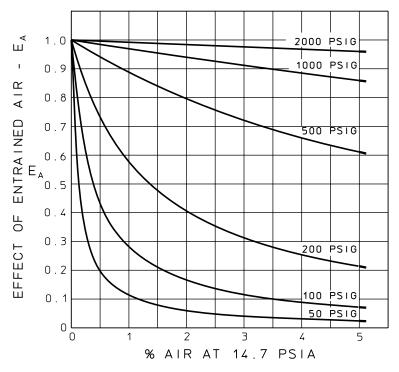
To simplify the calculations of thermal problems with entrained air, these curves show the *average* effect on a 230,000 psi bulk modulus for pressure points fairly close together. If a wide change in pressure is encountered in a problem, it would be more accurate to break the changes down into two or more steps, depending on the accuracy desired.
