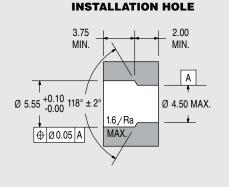
\* LOA before installation. All dimensions in millimeters.
