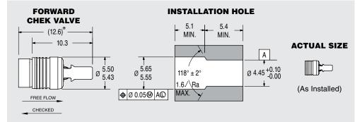
\* LOA before installation. All dimensions in millimeters.
