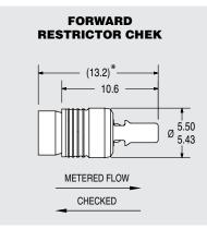
\* LOA before installation. All dimensions in millimeters.
