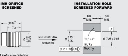
\* LOA before installation. All dimensions in millimeters.
