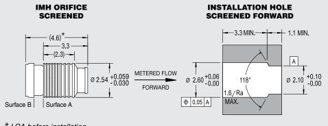
\* LOA before installation. All dimensions in millimeters.
