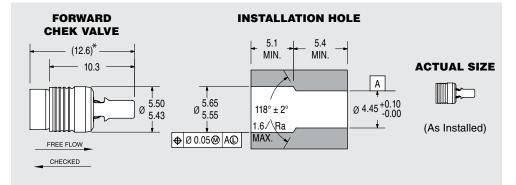
\* LOA before installation. All dimensions in millimeters.
