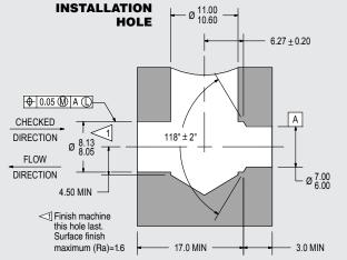
\* LOA before installation. All dimensions in millimeters.
