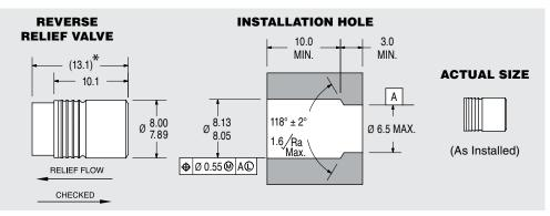
All dimensions are in millimeters. \* LOA before installation
