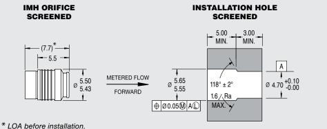
LOA before installation. All dimensions in millimeters.
