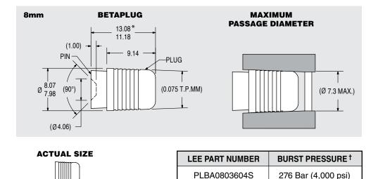
\* LOA before installation. All dimensions in millimeters.
