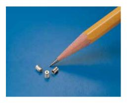
Installation is simple. Press or heat flow the orifice into a plastic hole, narrow end first, until the orifice is flush minimum with the top of the installation hole. Pressing or heat flowing the restrictors into the manifold or fitting provides retention and creates a leak tight seal.
