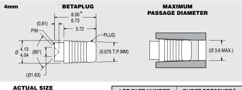
LEE PART NUMBER **BURST PRESSURE<sup>†</sup>** PLBA0402604S 483 Bar (7,000 psi) (As Installed)
