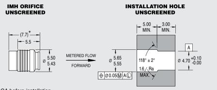
\* LOA before installation. All dimensions in millimeters.
