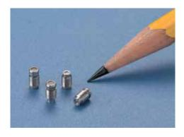
IMH orifices are so consistent because they are produced in high volume by automated processes. Installation is simple using the field proven controlled expansion principle which provides retention up to 21 mPa (3,045 psid) and creates a leak tight seal. Constructed entirely of stainless steel, these orifices will not change flow rate over time due either to corrosion or erosion. Integral safety screens are incorporated where the orifice diameter is 0.5mm (.020") or below.
